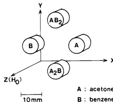
**Figure 1.** Two-dimensional test sample consisting of acetone (A) and benzene (B). A relaxation reagent, iron(III) acetylacetonate, was added so as to shorten the spin-lattice relaxation times down to about 100 ms for experimental convenience. Each cylinder has a diameter of 8 mm and a length of 10 mm. A, B, AB<sub>2</sub>, and A<sub>2</sub>B denote the constitutions of the solutions.
